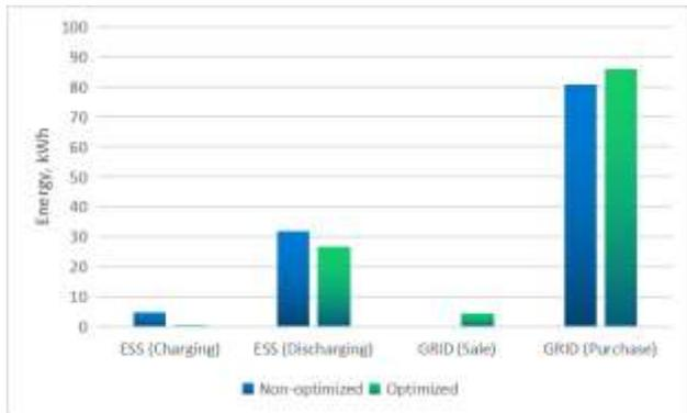
**Fig. 14. Comparison of energy dispatch for modes with and without optimization in winter**
